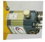
Detail of the exclusive hydraulic motor with integrated control valves
