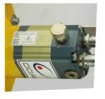
Detail of the hydraulic motor with integrated control valves
