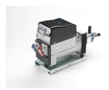
HW series are professional **DC** welders with capacity of 170 - 200 Ampere powered by hydraulic gear motor. The tools can be connected to the circuits of earth moving equipment, trucks, cranes, mobile workshops and all machines with sufficient hydraulic capacity.
